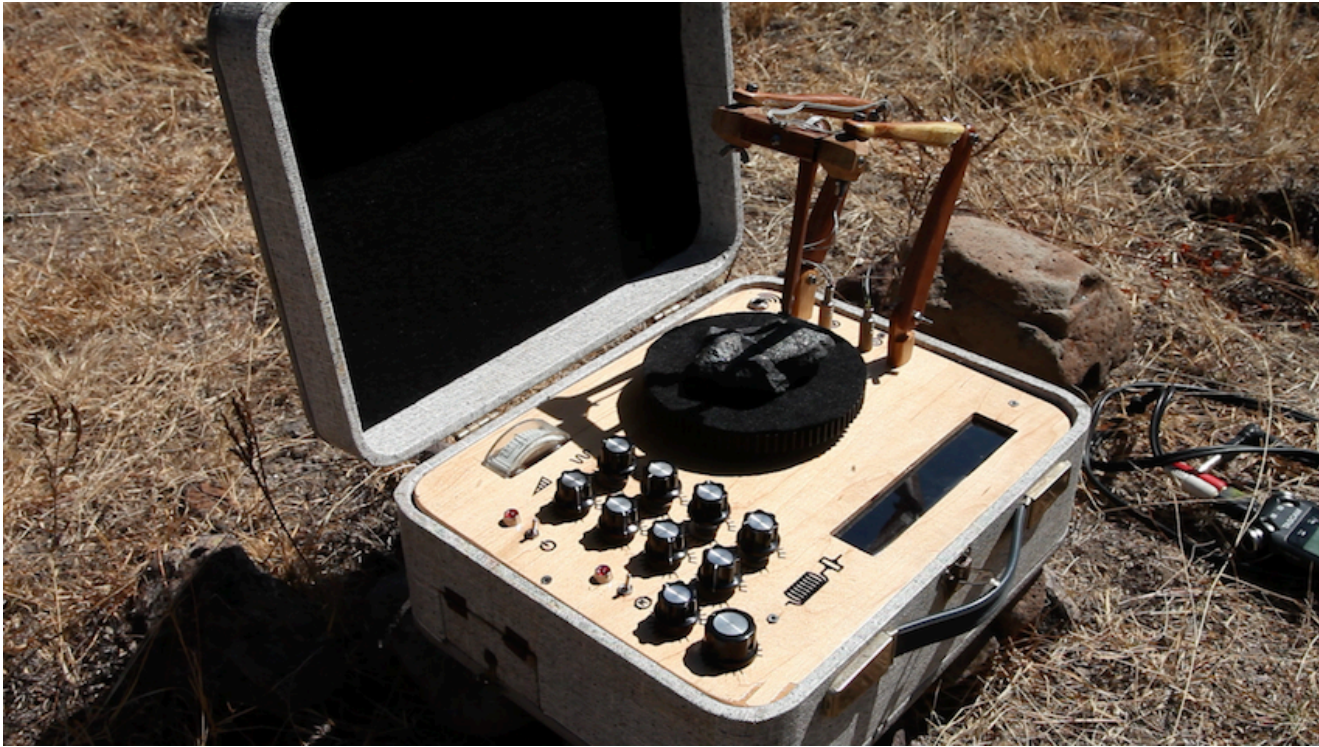
First prototype of Instrument to detect magnetic field of minerals and converting it into sound. Tsinamekuta Project.
